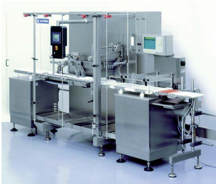
Image 1: CUT25 cutting machine from Alpma: Frequency converters and digital and analog IO are controlled synchronously with the control program via Profibus DP
