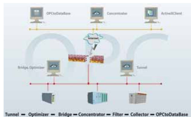
Fig. 4: Efficient data management in distributed systems with OPC, ODBC databases and MS Office products
