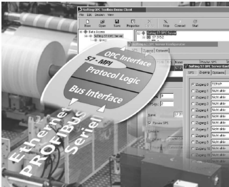
Figur 1: OPC can be used to conveniently access S7 and S5 controllers
