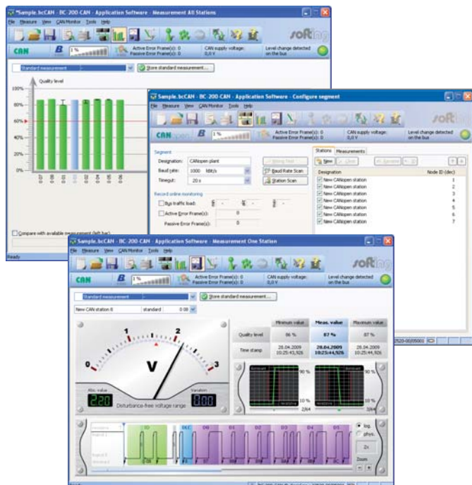
BC-200-CAN determines the signal quality on CAN based networks
