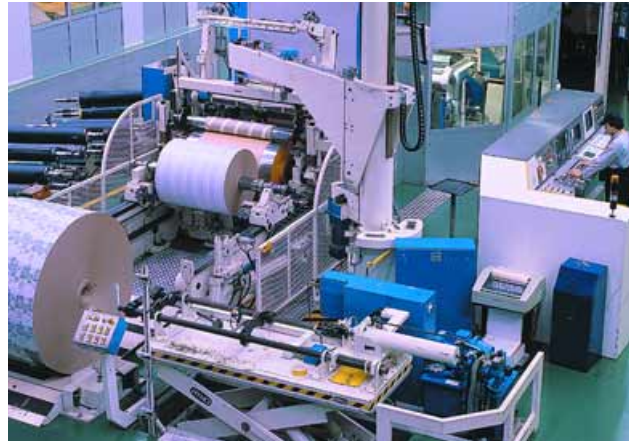
Production automation: PROFIBUS DP/V2 synchronizes high-speed drives with a precision of < 1 \mu\text{s}
